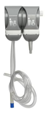
You will never have to deal with clogged metering tips with the INO jet proportioner. This problem was eliminated by switching to a system of controlling chemical dilution through a trough instead of an orifice. The trough is easily wiped clean, and there are four troughs per "metering peg" wheel for easy-to-adjust dilutions.
